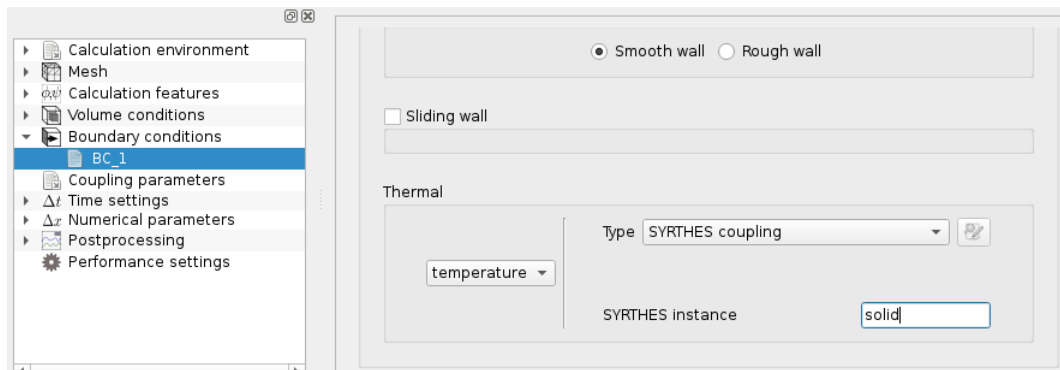
Figure 17: Boundary conditions - coupling with SYRTHES
