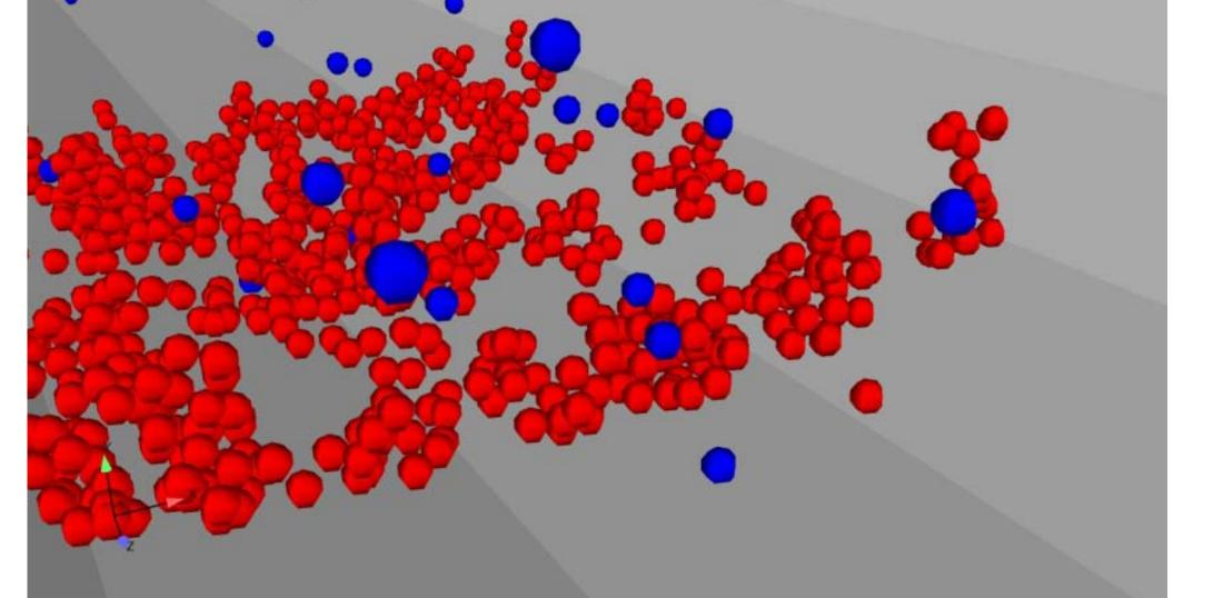
Different morphologies of the deposit (monolayer, dentrites, multilayer) can exist according to the chemical properties of the particles and wall.
