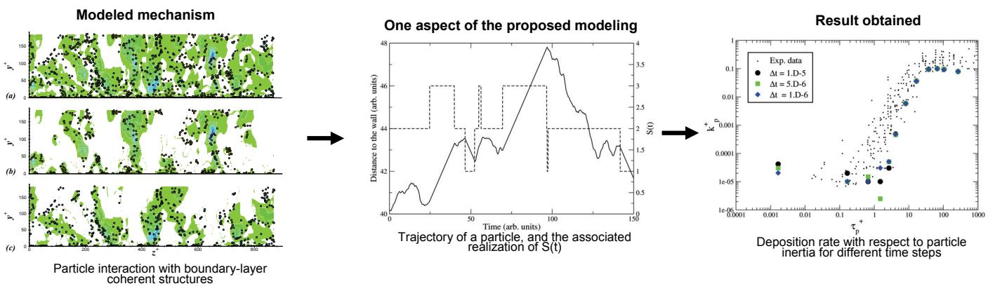
The model is first validated by comparing results obtained in the fluid-particle limit to available statistics of the boundary layer. Then, the deposition velocity is computed, and good agreement with experimental data is obtained. Furthermore, the two deposition regimes ("free-flight" and "diffusional") recently identified by DNS simulations are qualitatively retrieved.
