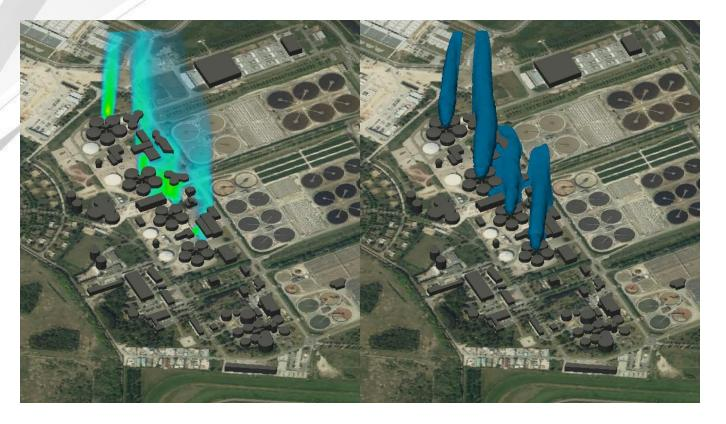
concentration at 1.5 m above ground level and 3D iso-contours (NOx)
