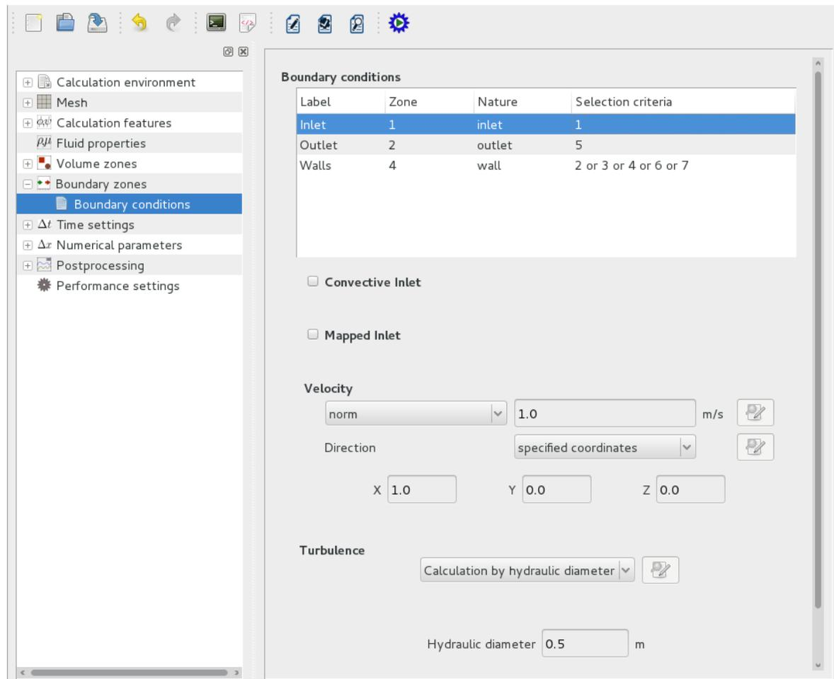
Figure III.23: Dynamic variables boundary conditions: inlet
