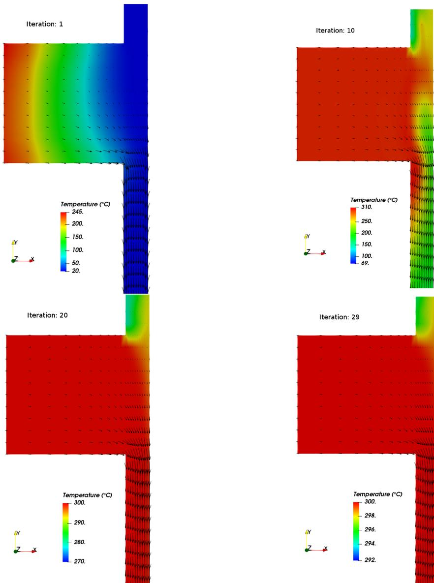
Figure II.5: Water velocity field colored by temperature at different iterations
