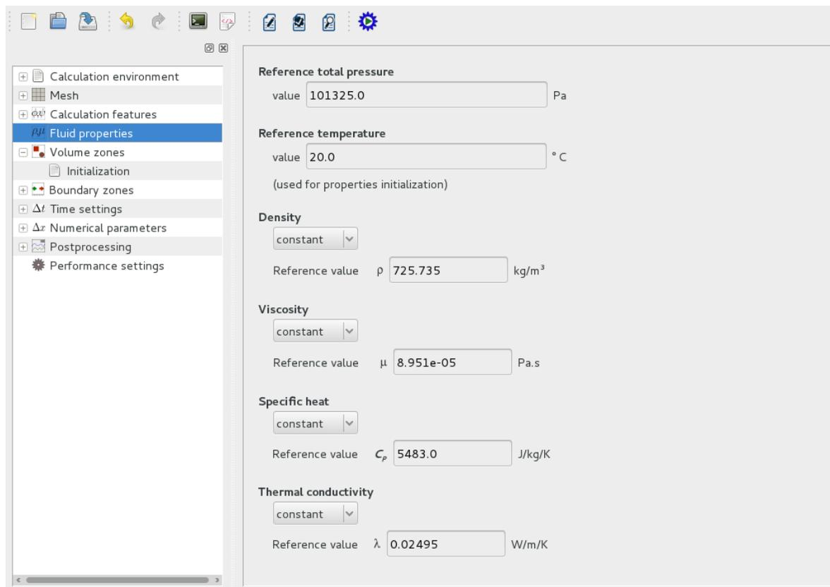
Figure III.15: Physical properties: fluid properties
