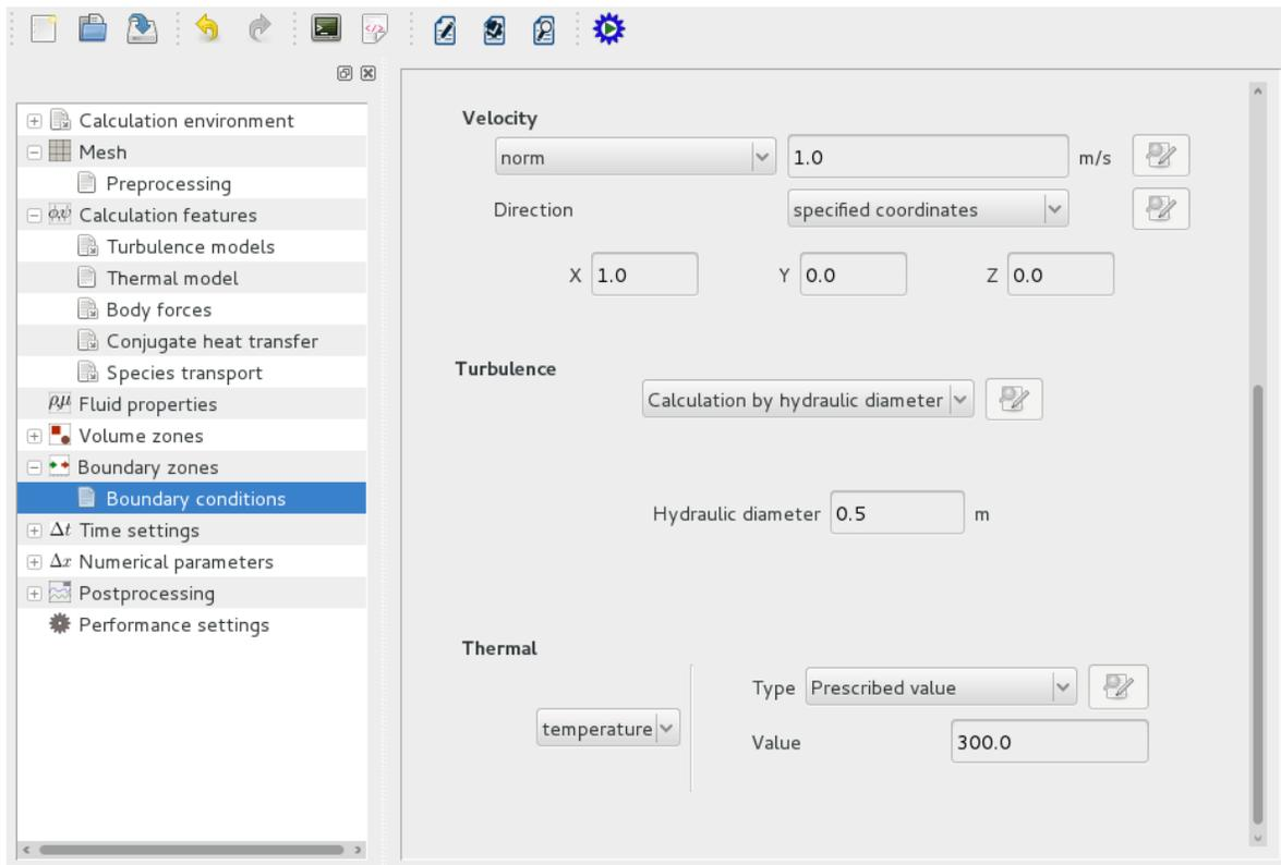
Figure III.24: Dynamic variables boundary conditions: inlet
