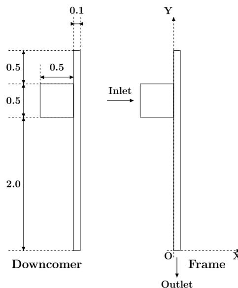
Figure II.2: Geometry of the downcomer
