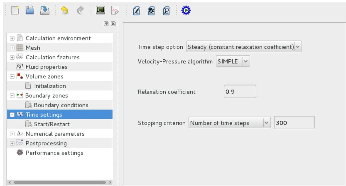
Figure III.27: Steady flow management
