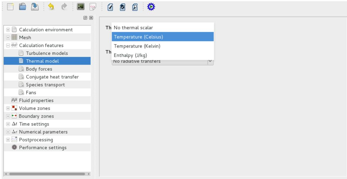
Figure III.8: Thermal scalar conservation: list of models
