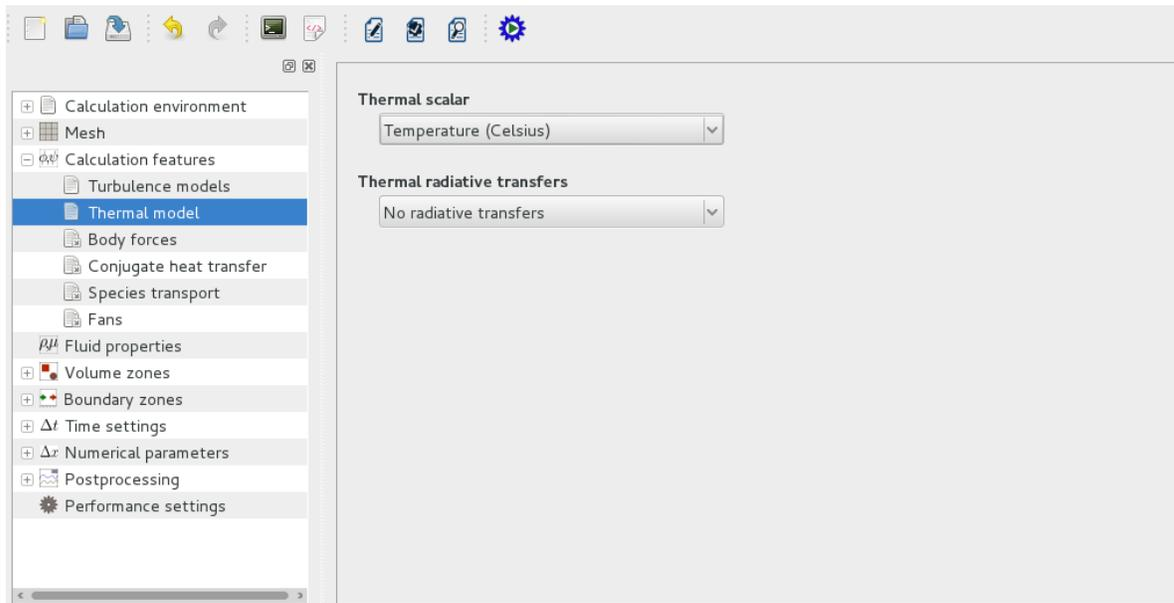
Figure III.9: Thermal scalar conservation: choice of a model
