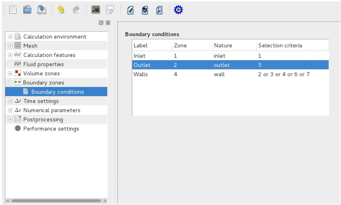
Figure III.22: Dynamic variables boundary conditions
