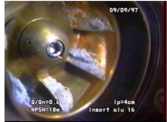
Cavitation pockets on rotor blades
