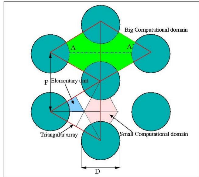
Sketch, of the rod bundle geometry where  $D$  is the diameter of a fuel pin and  $P$  is the distance between the center of two adjacent fuel elements (pitch). In this study the small computational domain (pink) was used.
