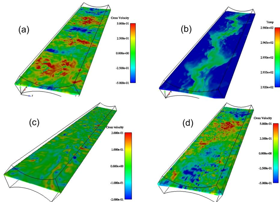
Instantaneous flow fields in the mid plane A-A' : Cross velocity  $W$  (a) and temperature (b) (LES6K); (c) Cross velocity  $W$  (LESWPD); (d) Cross velocity  $W$  (HYB6K). In (a) and (d) an alternative pattern positive and negative of the velocity is very clear, meaning a strong exchange between sub-channels. This phenomenon is not visible in figure (c). The results of the flow fluctuations is a meaning temperature field (b)
