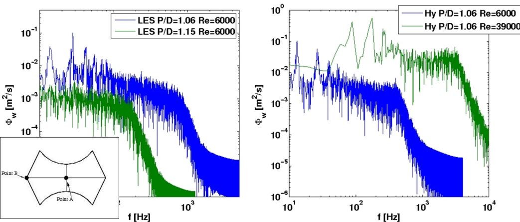
Power spectra in time of the velocity fluctuation ( $w$ ) in the azimuthal direction. The probe is located in the centre of the domain (point A of the small adjacent picture). The spectra, for the tight geometry, are characterized by two dominant frequencies and the dimensionless value are reported in table below
