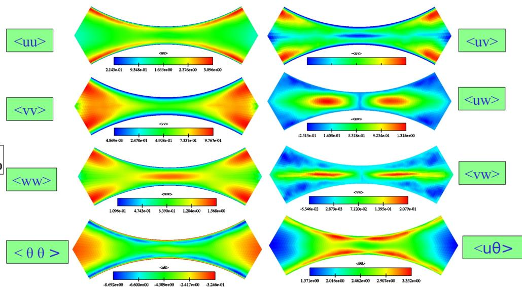
Adimensionalized mean Reynolds stresses for the case LES6K. It is interesting to notice that for  $\langle ww \rangle$  the maximum, in the gap region, is located in the middle of the geometry. This is a clear consequence of the flow fluctuations in the area.
