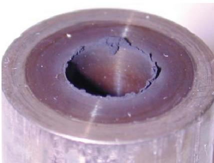
Fig. 4 : Observation of the deposition on the leading edge of the sudden contraction on EMILIE (experimental loop at Areva-NP-Centre technique).
