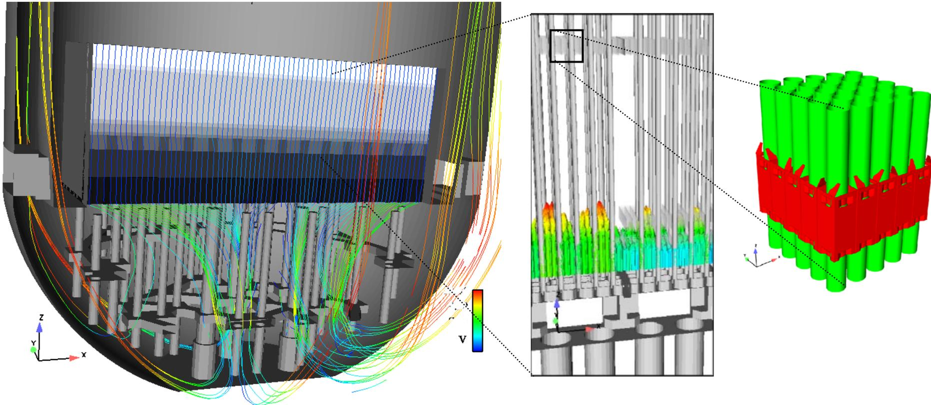
Lower part of 1300 MW core vessel
