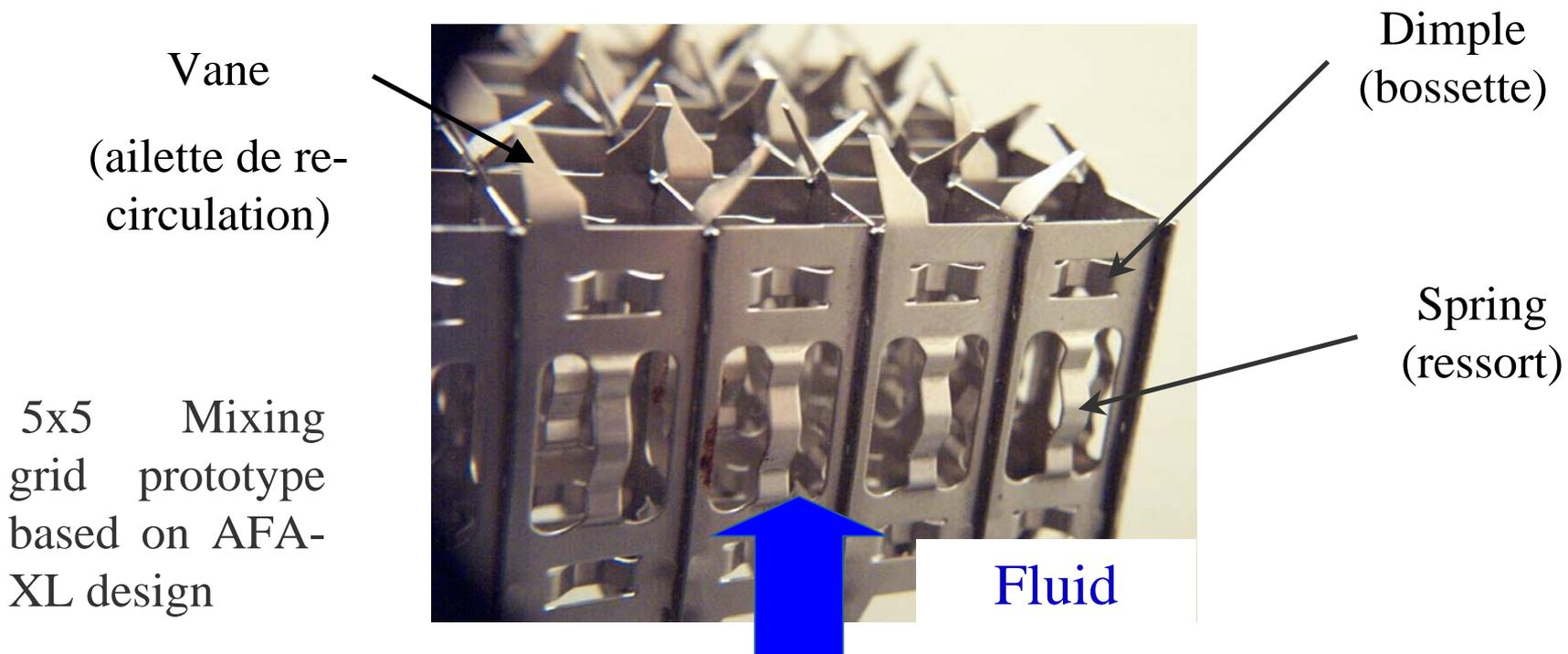
A specific design for each type of mixing grid
