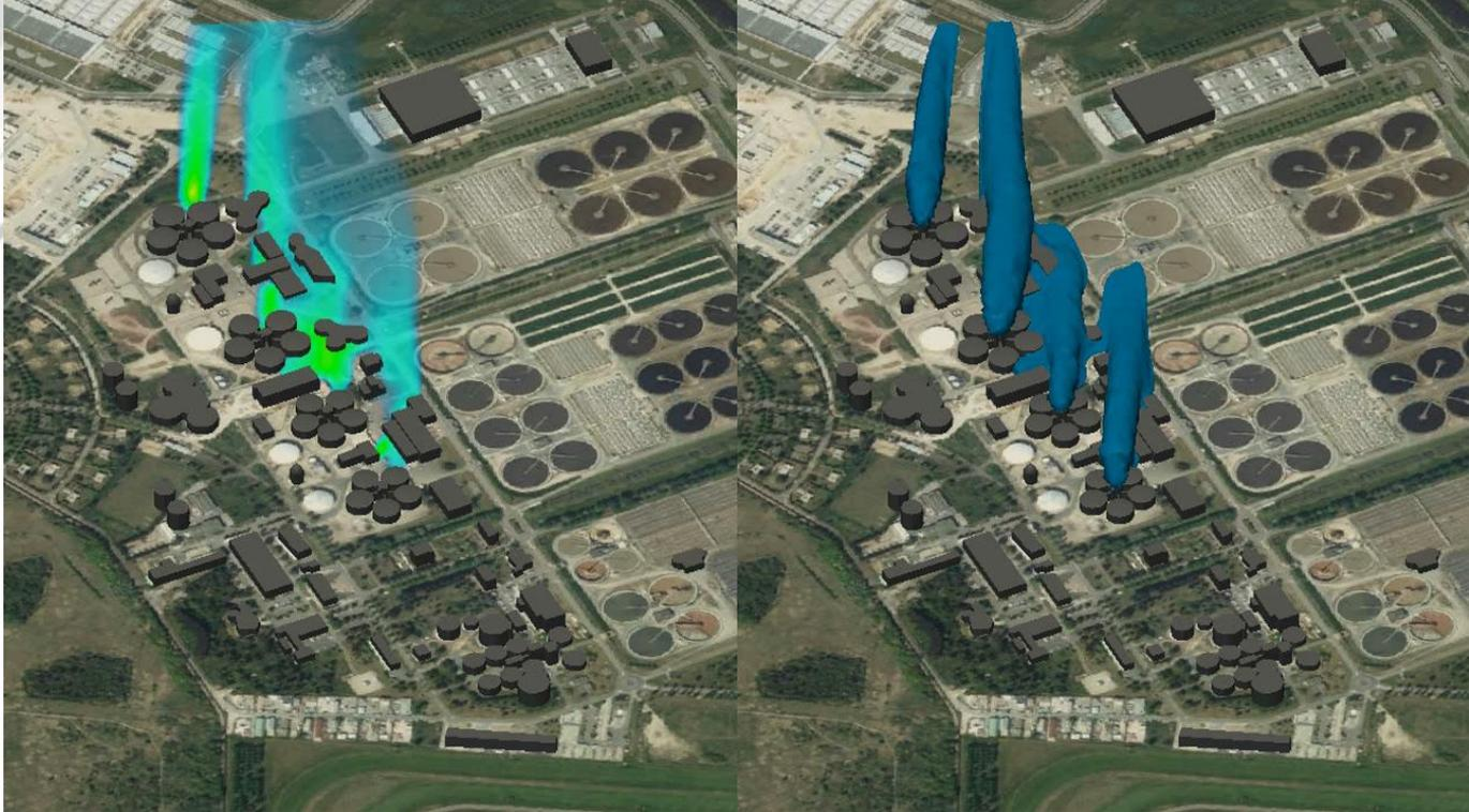
concentration at 1.5 m above ground level and 3D iso-contours (NO<sub>x</sub>)
