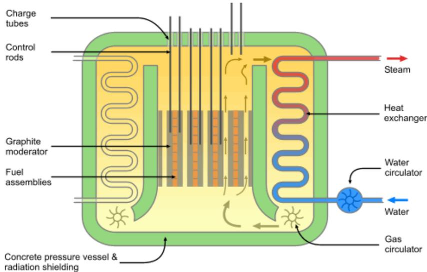
Schematic diagram of the AGR core
