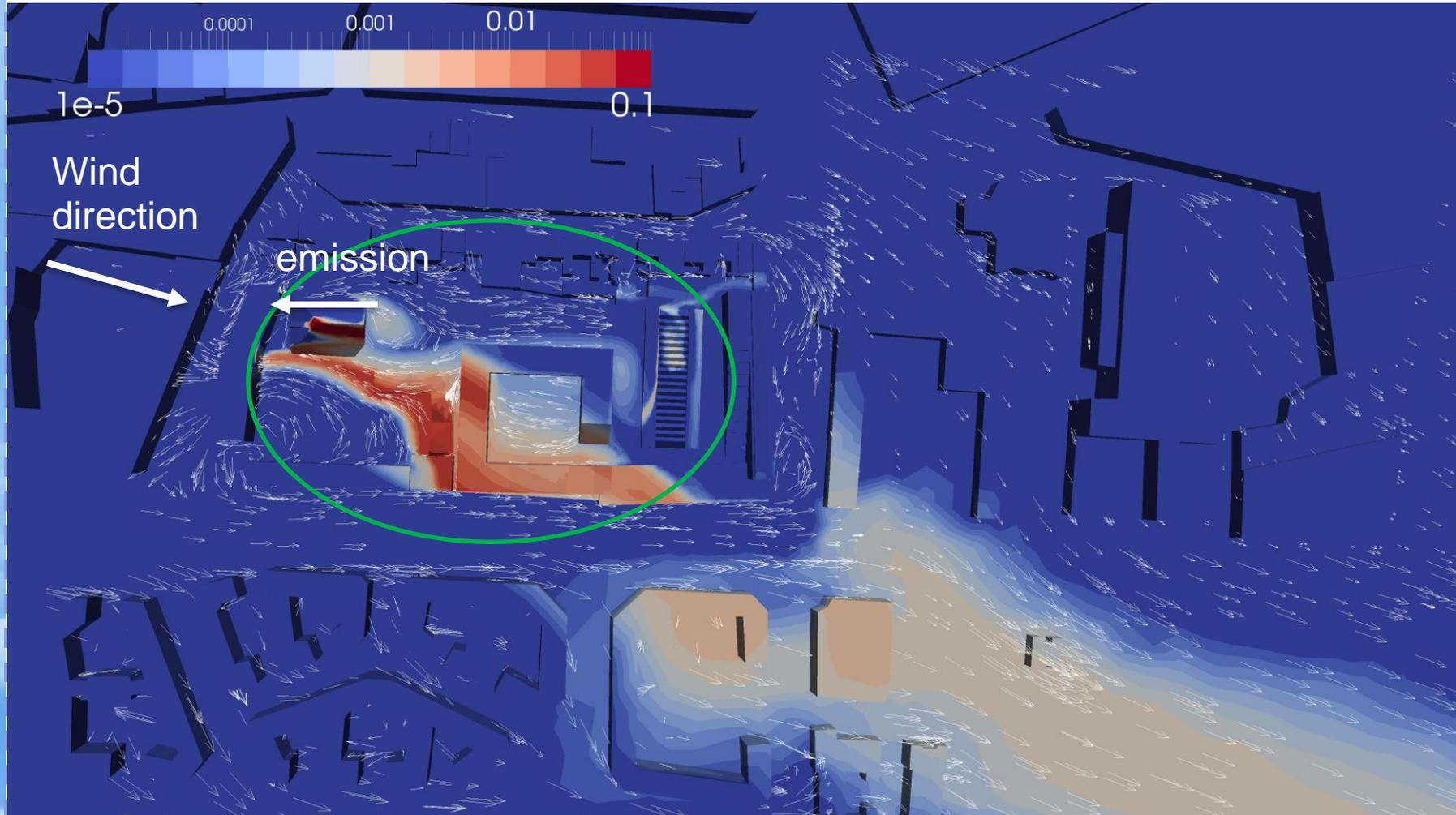
*Concentration field near the ground and near the walls of buildings – Velocity vectors field projected at  $z = 12m$*
