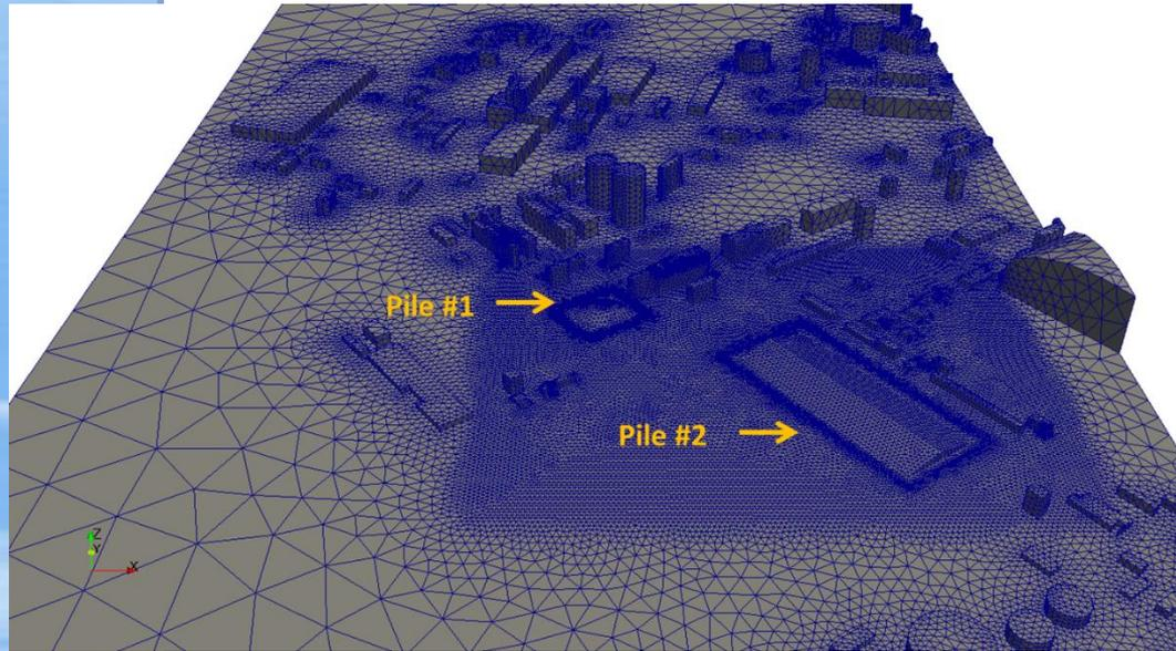
The meshes are also computed with Salome using tetrahedron elements and 2 zones for refinement.
