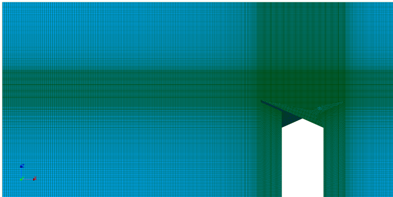
Figure: PK Weir - Mesh of the domain (min. cell size 5cm)
