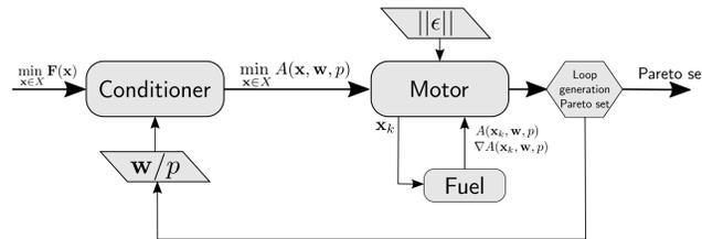
Figure 2: Optimization chain: *Code\_Saturne* and SYRTHES included into Fuel module.
