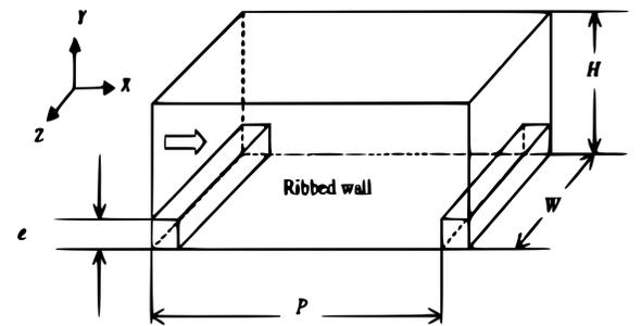
Figure 3: Case dimension:  $H = 50$  mm,  $W = 50$  mm,  $e = 7,5$  mm et  $p = 12e = 90$  mm.
