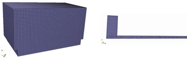
Figure 4: Structured mesh for the fluid domain and unstructured for the solid domain.
