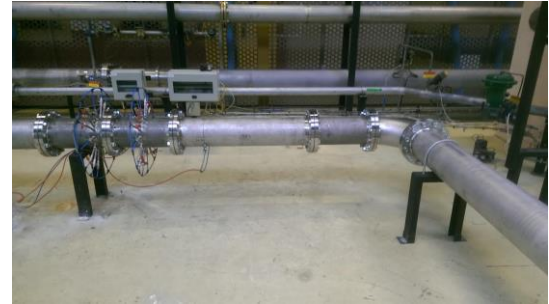
ex. Single 90° bend with no minimum straight lengths in the upstream side
